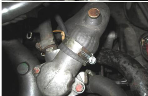
You can also see in the lower photo, the blanking plug now fitted on the right hand side of the thermostat housing. This is the position where the new engine temperature switch for activating the fan, will fit. It has exactly the right thread (M14 x 1.5mm) for these switches! The one you want has a 95/90°C setting. At the same time the radiator switch should be changed for a 92/87°C switch. This will allow for the approximately 3°C drop between the engine and radiator.
