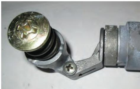
these were an early and later design, although I can't confirm that. What I do know is that if the design on the right in the picture above, is fitted, you have to be more careful about folding the mirror head, when moving it out of the way.
