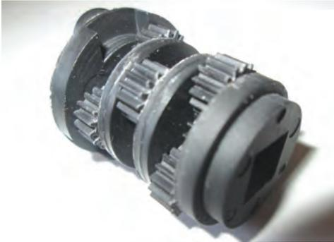
*Two views of the epicyclic gear assembly, with the square hole on the last carrier in the lower shot*
