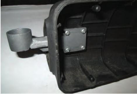
Above: Mirror head mounting casting (with rubber bellows removed) and Below: broken casting
