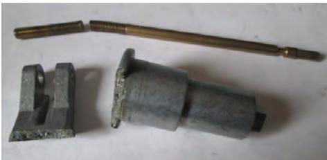
part in the system and that is because the alloy casting is so porous its many bubble holes weaken it, and the cross sectional area is too small for the load it has to take.
