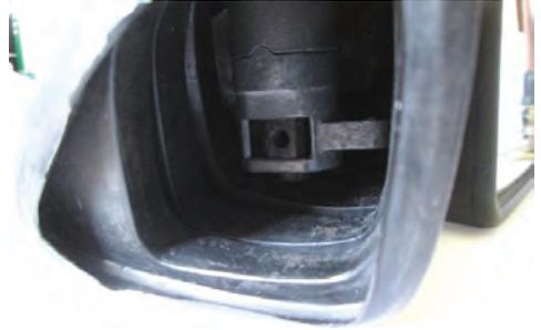
The view into the mirror rubber bellows should look like that above. You screw the end of the new rod into the plastic block. As you screw it in, the open jaw of the new alloy piece will reach a point where it will fit over the pivot arm, the holes will align and you can put the screw back in to the jaw and mirror head pivot arm to secure them together. This job is a little tricky as the rubber bellows tends to get in the way, but if you push it back you can do it.
