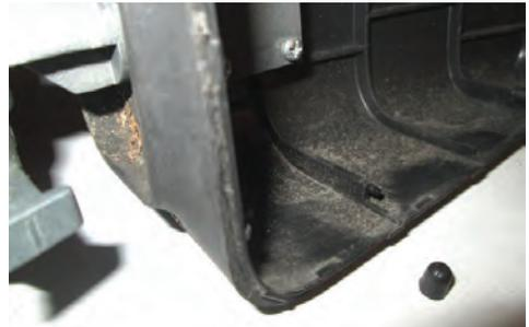
The glass sits on four rubbers that fit on four pins in the head moulding, (*see above*) so if the glass is already missing, check if these small rubbers are still there as you will need them. If the glass is fitted but rattles or can be moved in the head shell it is likely these small rubbers are missing.
