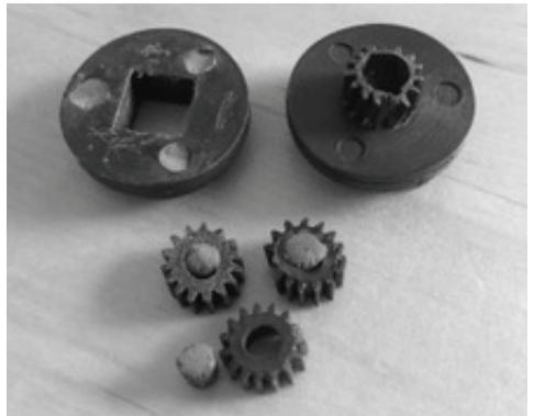
*Note that some of the gear teeth are broken both on the carrier central one as well as the individual ones*
