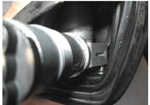
The photo at the bottom of page 8 shows the screw in but not yet secured. The screw should have a spring washer fitted to keep it secure from coming undone, but as it is a pivot the screw should not be so tight that it stops the mirror pivoting in and out.
