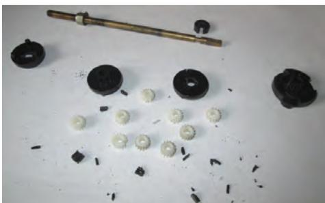
*Broken gear mechanism from inside barrel*
