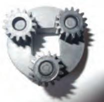
You rotate the knob which turns the first central gear and that rotates the mating three gears, which turns the first carrier which then turns the next three gears and therefore that second carrier and the central gear on that carrier turns the final three gears on the last carrier which has the central drive square hole.
