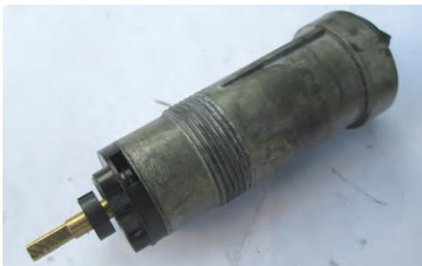
Once the rod is out, you can strip the remaining parts out of the tube. Have a nice clean area for these pieces to go on so you can see them all clearly. If the mechanism is broken, it may look like this:
