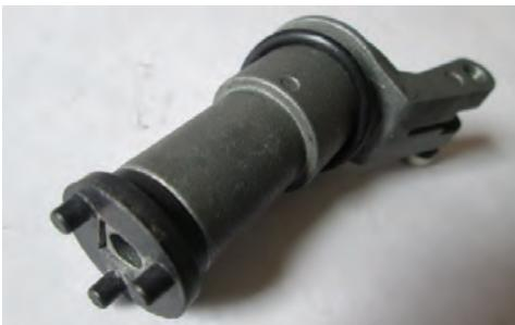
You can only turn this mechanism with its 64:1 ratio, from inside the car. It can't be reverse rotated from outside and if you tried to do that, something will break.
