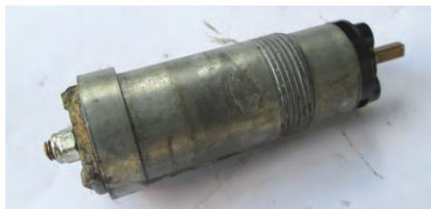
To strip this, you need to undo the Nyloc nut off the remains of the rod, and push the rod out of the other end. If the rod is not broken you only need to undo the nut back about 6mm and push the nut up to the body which will expose the thick 'U' shaped clip at the other end, which was in the carrier recess. (*next photo*) Now remove the 'U' clip from the rod and push the rod with nut out the opposite end.
