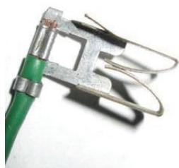
at the ends and the curved 'tails' are designed to grip the board with the 'tails' on the bottom having positive contact with the circuit board contact patches. The problem is they crack across those end bends and lose firm grip on the board. They might look OK in the plug housing at first glance, but check them with a small screwdriver.
